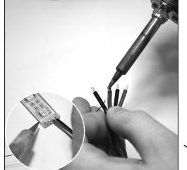
Use the soldering iron to tin the wires on the Covelight Superior RGBW; The Brown wire comes on the +24V connection The red wire comes on the R connection The green wire comes on the G connection The blue wire comes on the B connection The white wire comes on the W connection
