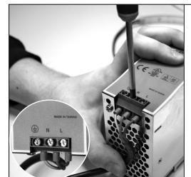
At the end of the power cable, fit the crimp terminal over the stripped wires and fixate the crimp terminal.
