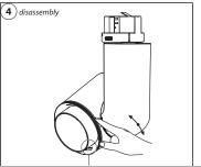
Removing the snoot: rotate the accessory holder
