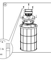
ļ ATTENTION Make sure the gasket & parts are dust, mud and sand free to ensure the IP67 classification when mounting the RVS ring back on the REVO Inground!
